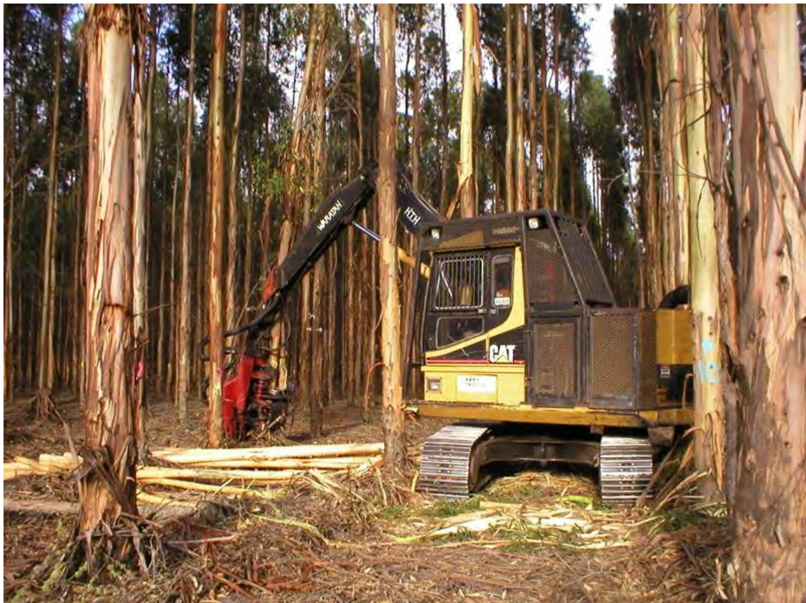
Figure 35. Caterpillar 320: tail swing causing considerable difficulty perpendicular to the direction of travel.
