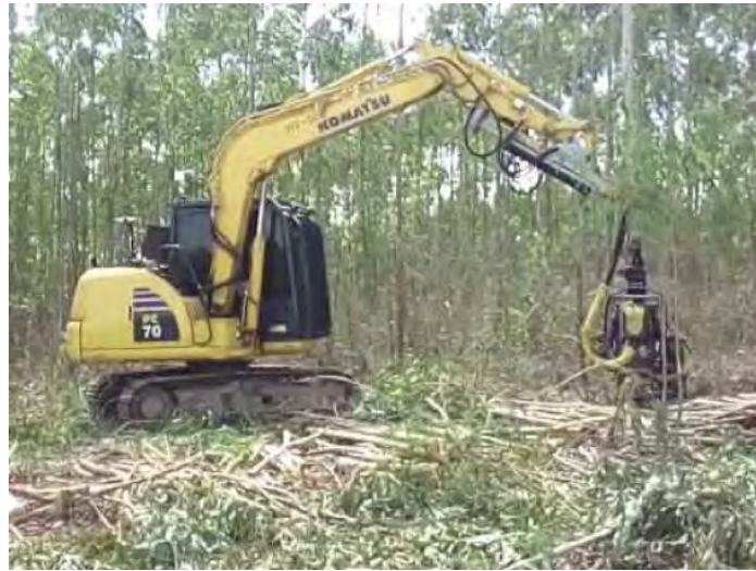
Figure 8. Komatsu PC70 6.5 tonne excavator with harvesting head
