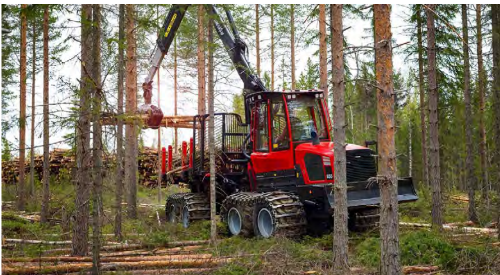
Figure 54. Komatsu 855 Forwarder (14 tonne)
