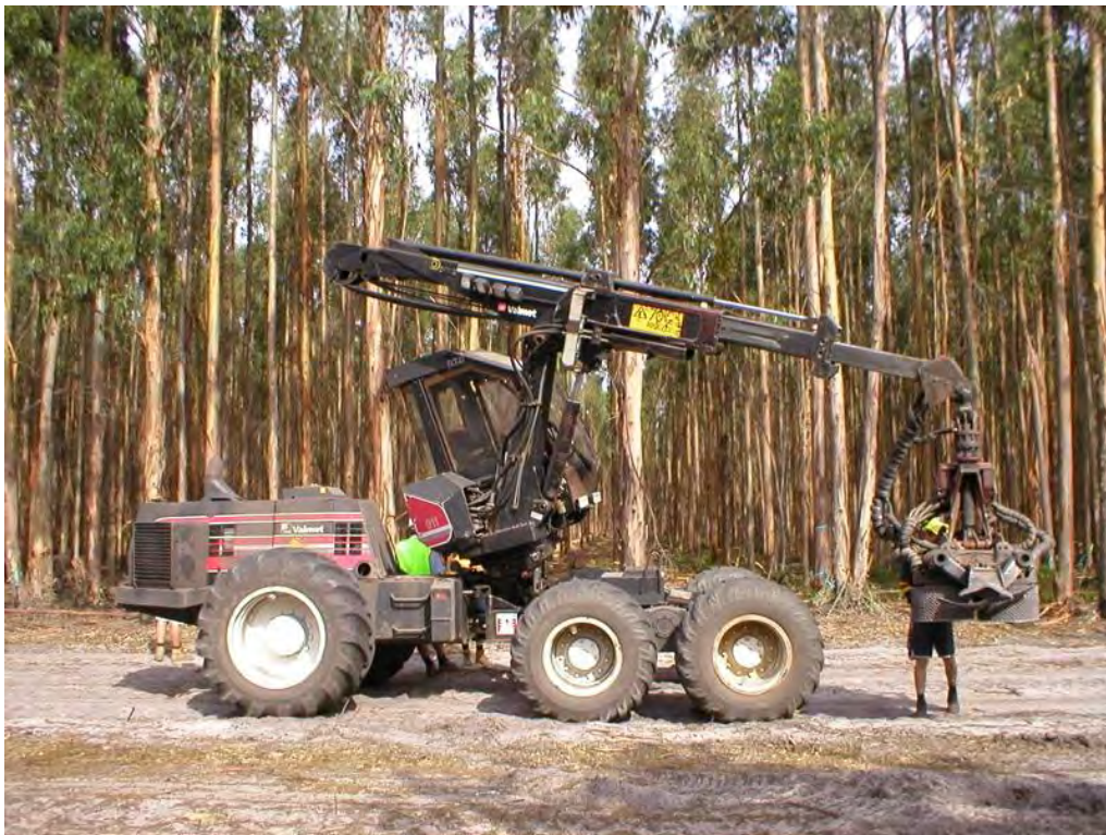
Figure 25. Valmet 911 with Valmet 965 harvesting head
