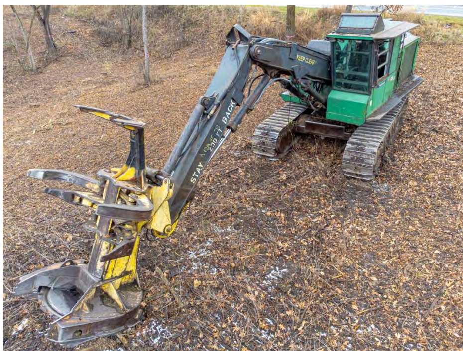
Figure 18. Feller buncher with continuous circular 'hot' saw
