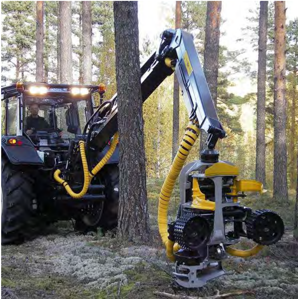
Figure 16. Small forest harvesting head 350kg by Kesla
