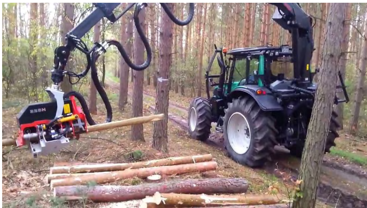
Figure 7. Valtra tractor adapted for tree harvesting
