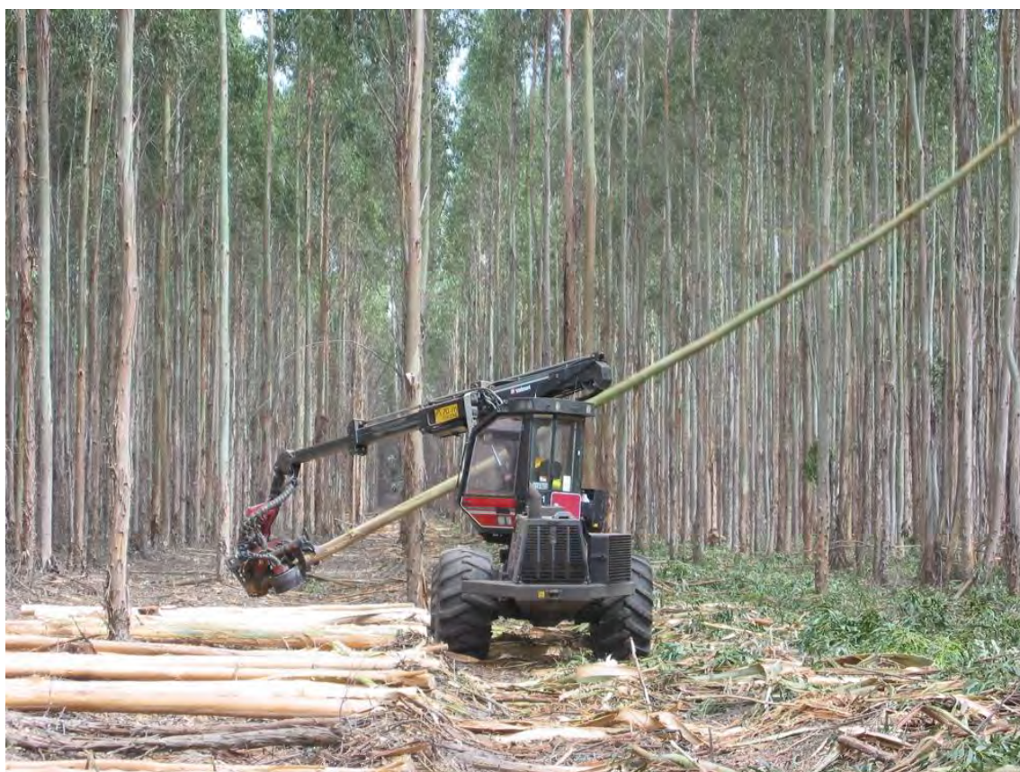
Figure 36. Valmet 911 with no tail swing when working perpendicular to the direction of travel.
