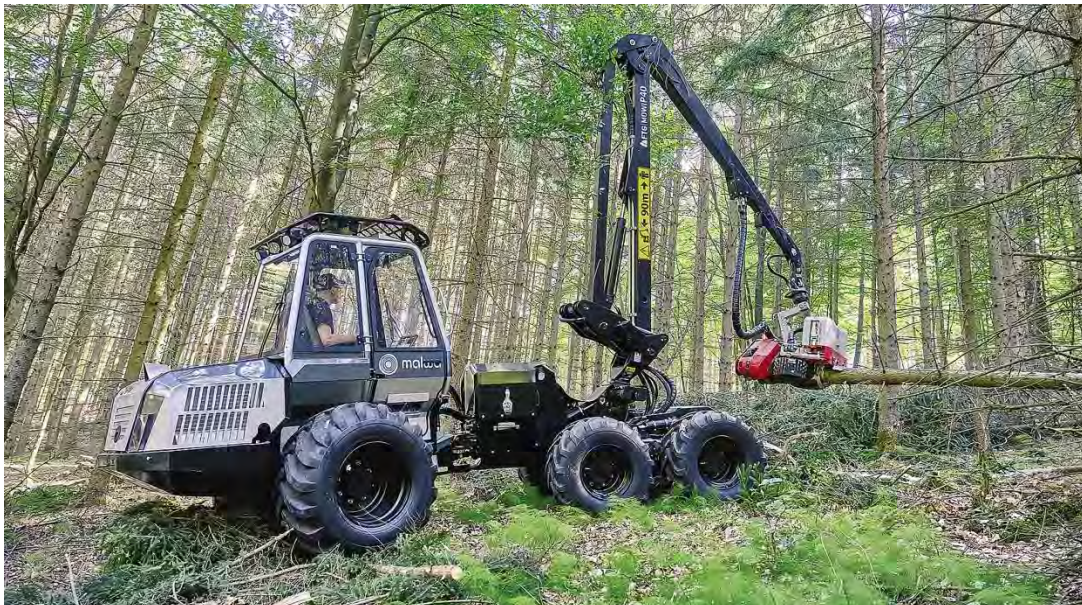
Figure 9. Malwa 560H 5.7 tonne purpose-built harvester.
