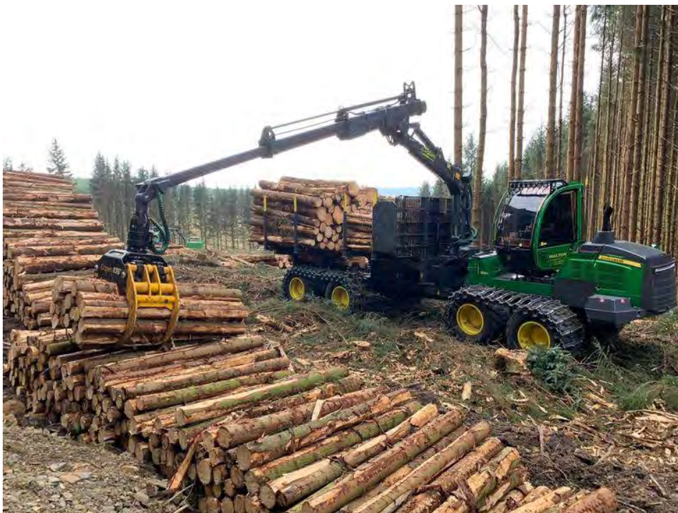
Figure 12. John Deer 1510G forwarder 15 tonne load capacity
