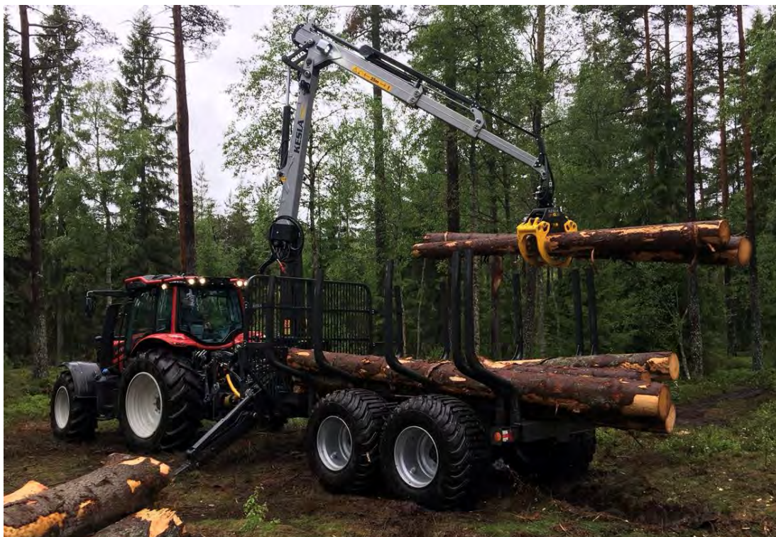
Figure 13. Valtra reverse-steer tractor with forwarder trailer
